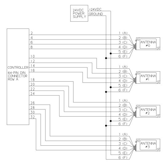
Note: Connections to Antennas 1, 2 and 3 Apply Only When Using the HS850B-4 Controller.
